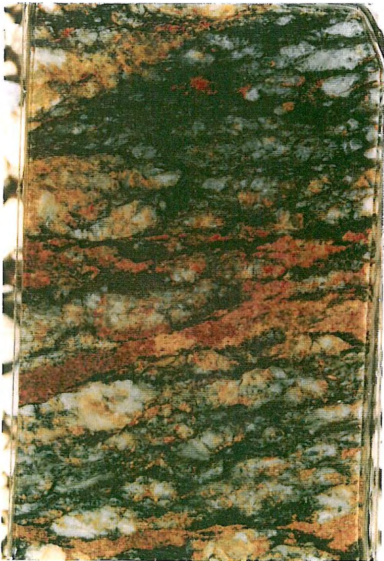
WCP37 470'/00023/07/DAY/3X/KBX MIXED CATACLASITE showing typical appearance of hand specimen. Reddish domains are calcite (M13), light colored domains are altered quartz diorite (E9-G9), and dark colored interstitial domains are metapelite (M3, G15).
