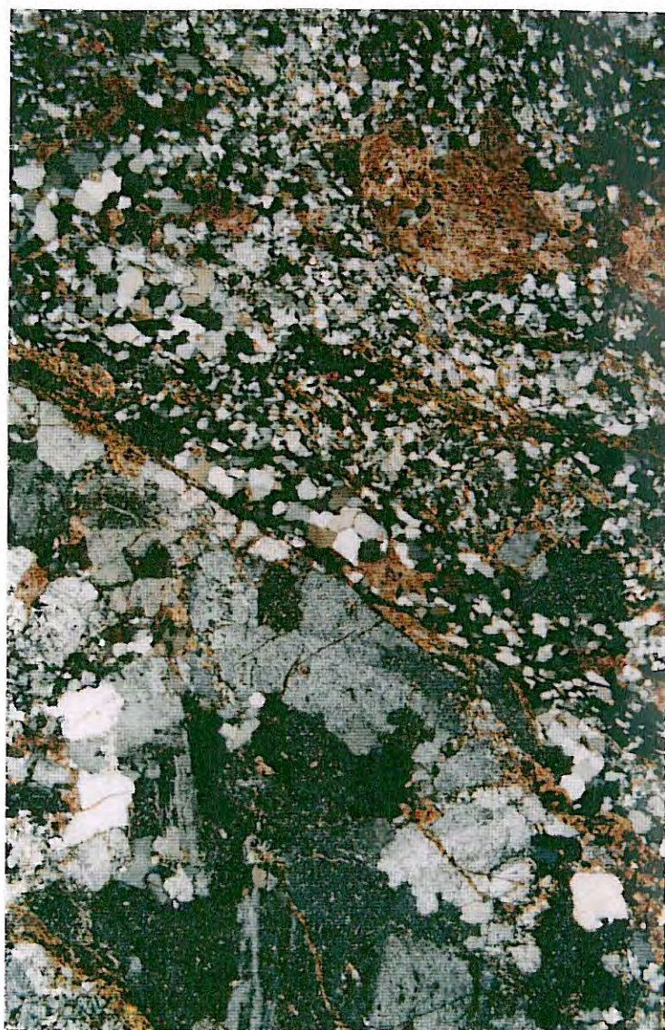
WCP37 470'/00023/23/XPL/28X/KBX MIXED CATACLASITE showing typical appearance of interlensed [altered quartz diorite (A1-J13) + metapelite (I15-T30)].
