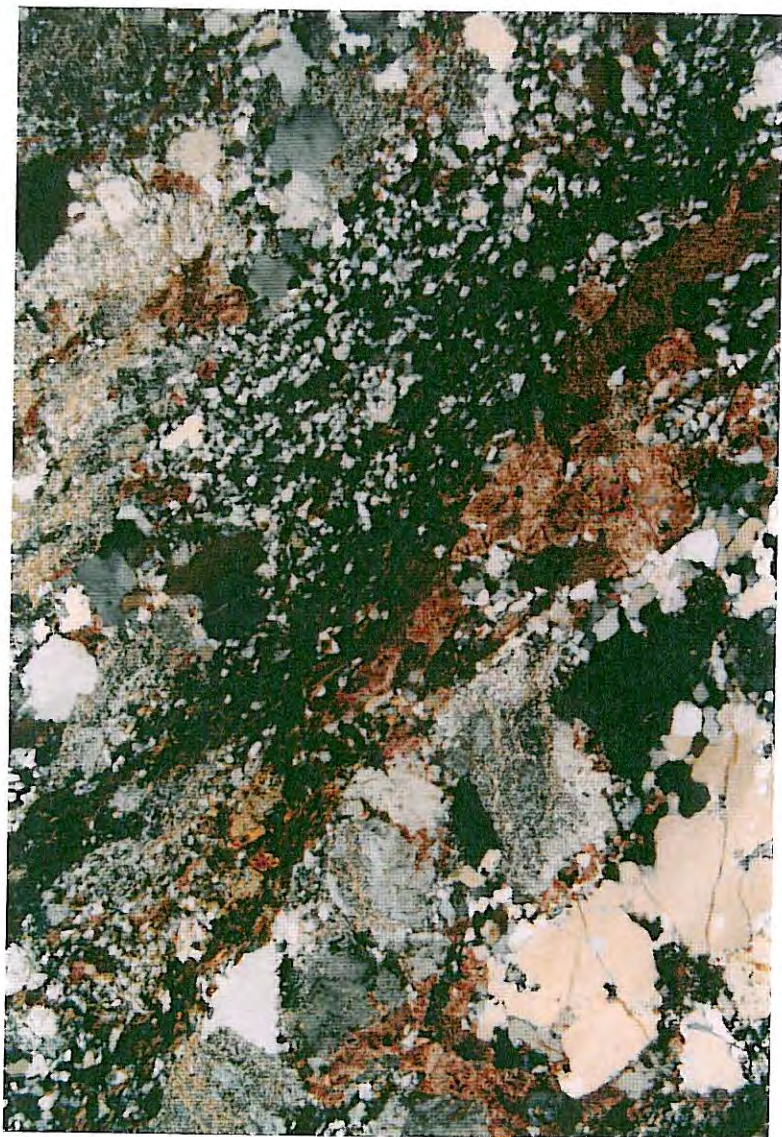
WCP37 470'/00023/22/XPL/28X/KBX MIXED CATACLASITE showing typical appearance of interlensed [altered quartz diorite (L1-T11) + metapelite (J18-T26)].
