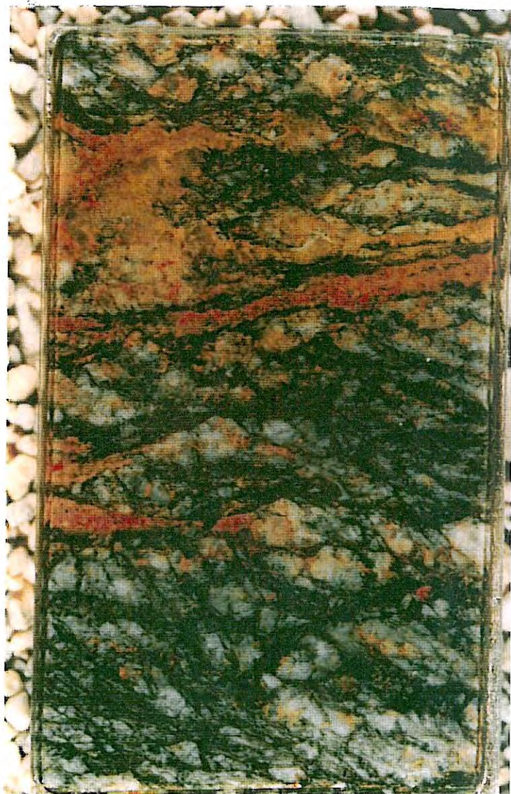
WCP37 470'/00023/08/DAY/3X/KBX MIXED CATACLASITE showing typical appearance of hand specimen. Reddish domains are calcite, light colored domains are altered quartz diorite, and dark colored interstitial domains are metapelite.
