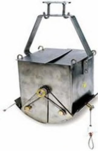
FIGURE 2 - Example of an Ekman™ Dredge
