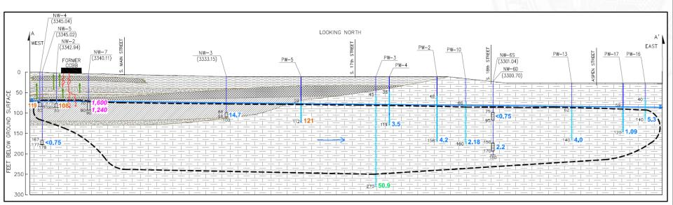
LEGEND PCE CONCENTRATIONS IN ug/L MVH-2 WELL IDENTIFICATION GRAVEL AND SAND LIMESTONE/MUDSTONE VAPOR TRANSPORT 430 27 < 50 300 - 500 TOP OF GROUNDWATER TABLE (APPROXIMATE) SAND SILT 740 98 700 - 1,000 50 - 100 PCE TRANSPORT PATHWAY 120 WELL SCREEN INTERVAL OPEN HOLE SILTY CLAY 1.200 160 100 - 300 > 1,000 AND 165 PRIVATE WELL AND APPROXIMATE EXTENT OF TOTAL DEPTH OF WELL TOTAL DEPTH OF WELL IMPACTED GROUNDWATER 158 185
