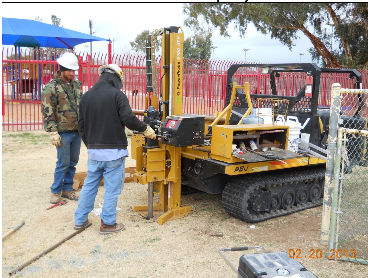
Installing temporary soil gas probes in Gollob Park, Gollob-2013-2 (Feb 20, 2013)
