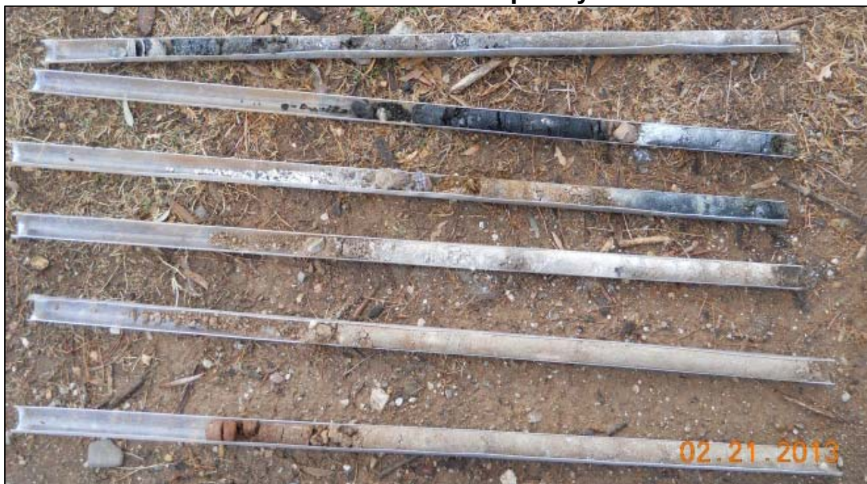
Acrylic liners with material removed during probe installation, Gollob-2013-4 (Feb 21, 2013)
