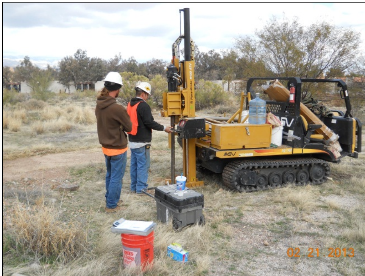
Shallow temporary soil gas probe installation (February 21, 2013)
