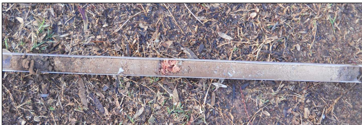
Acrylic liners with material removed during probe installation (February 21, 2013)
