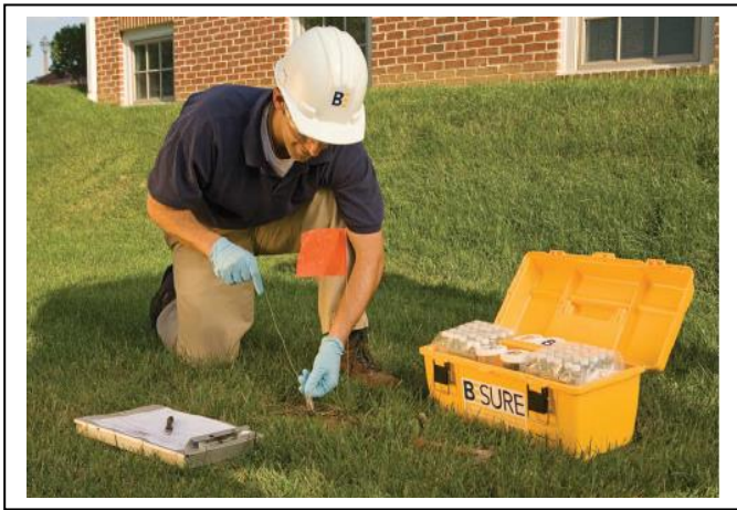
Figure 6.20 Installation of a passive soil vapor sampler (Beacon-USA.com)
