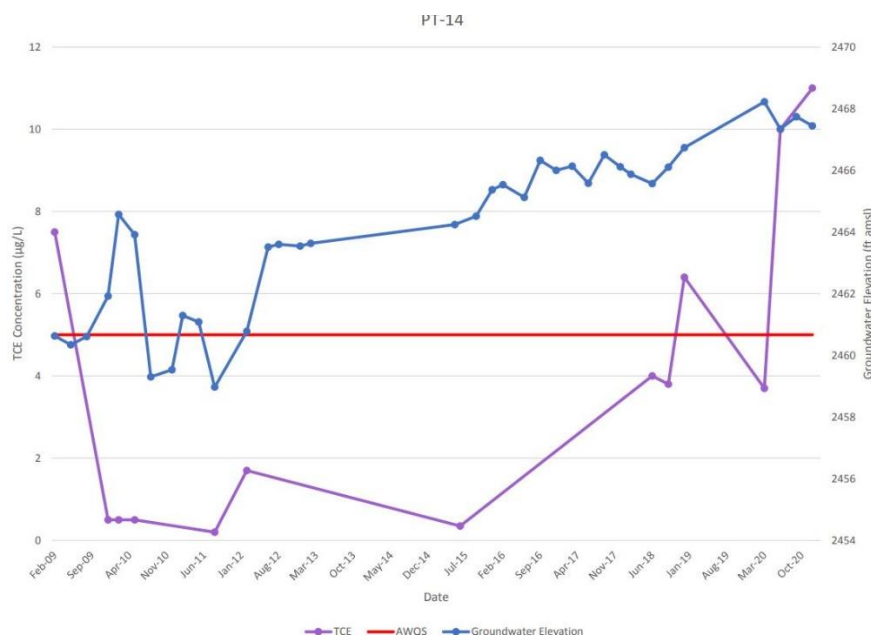
Figure C14 TCE Concentrations and Groundwater Elevations at PT-14 Lower Unit
