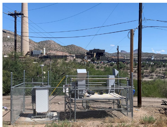
Hillcrest Pb samplers and stand. The ASARCO stack is in the background – 09/2019
