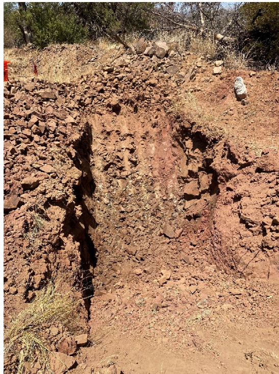
Photo 8 – TP21-05 – Test Pit terminated due to bucket refusal at shaft platform
