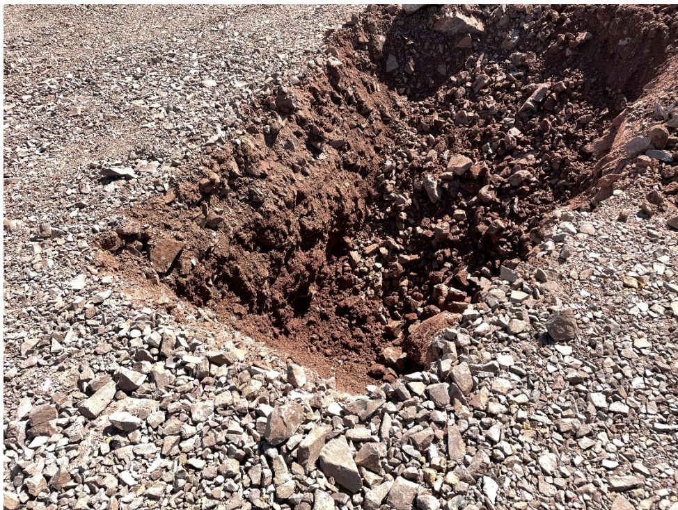
Photo 10 – Test Pit (WTP2 material stockpile at the IP)
