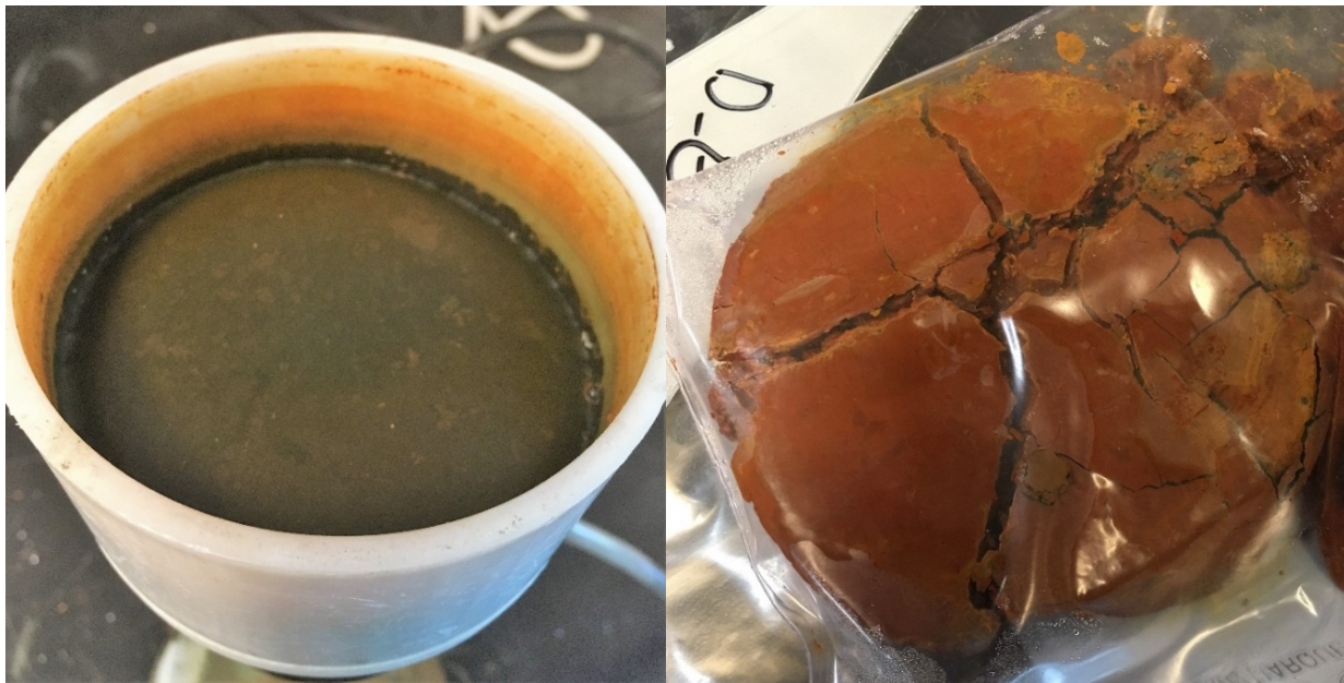
Figure 5-5 Thickened and filtered solid residue samples generated during the ERC tests.
