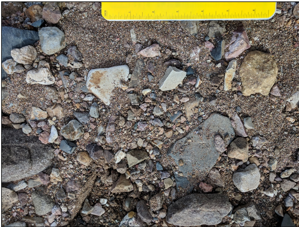
Figure 2 – Sample Input Photograph to Determine Sediment Gradation using FHWA’s Hydraulic Toolbox (Site 2 pictured)
