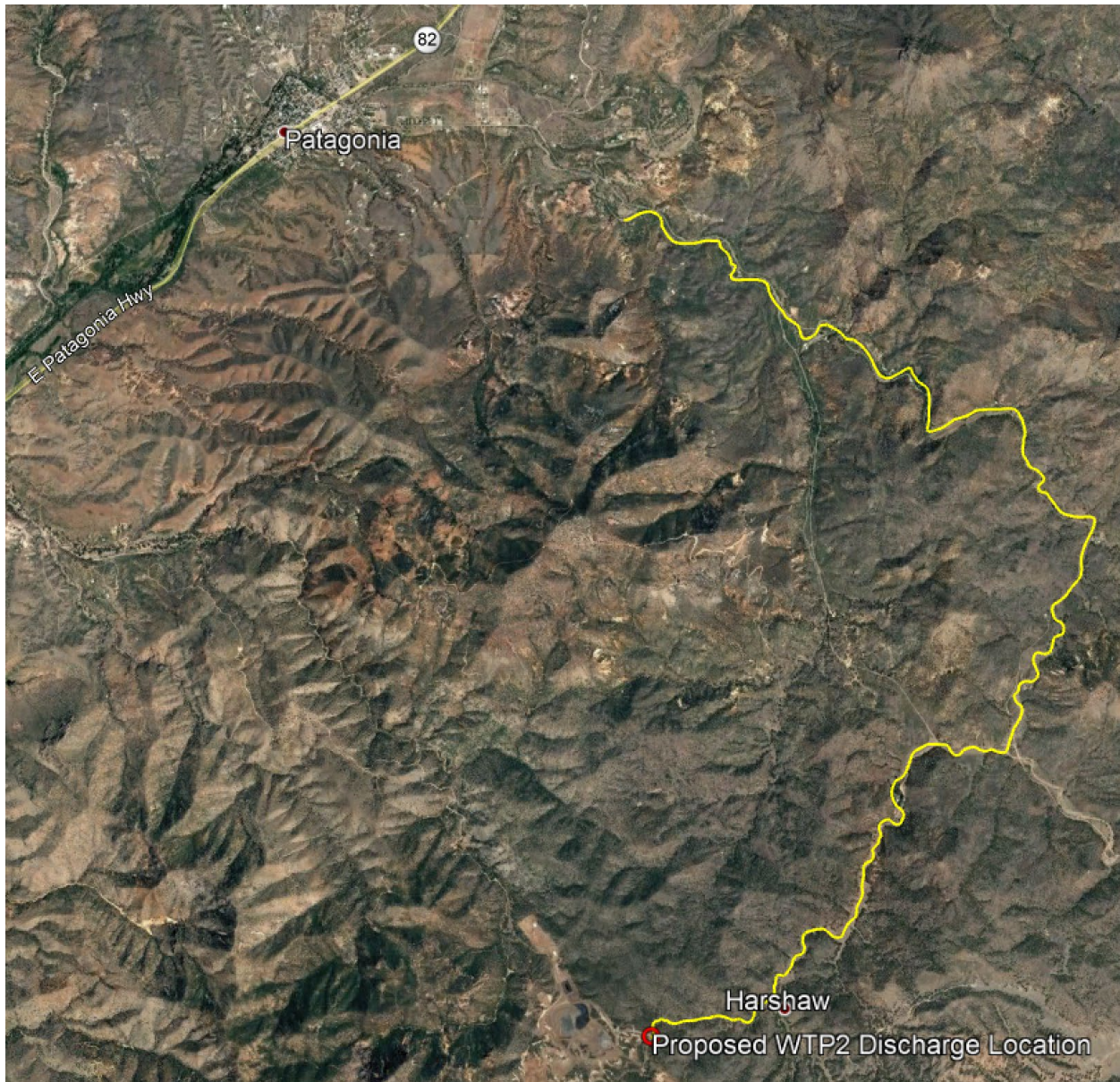
Figure 11 – Extent of Calculated PMA in Harshaw Creek (yellow) Resulting from Maximum 4,500 gpm Discharge from WTP2
