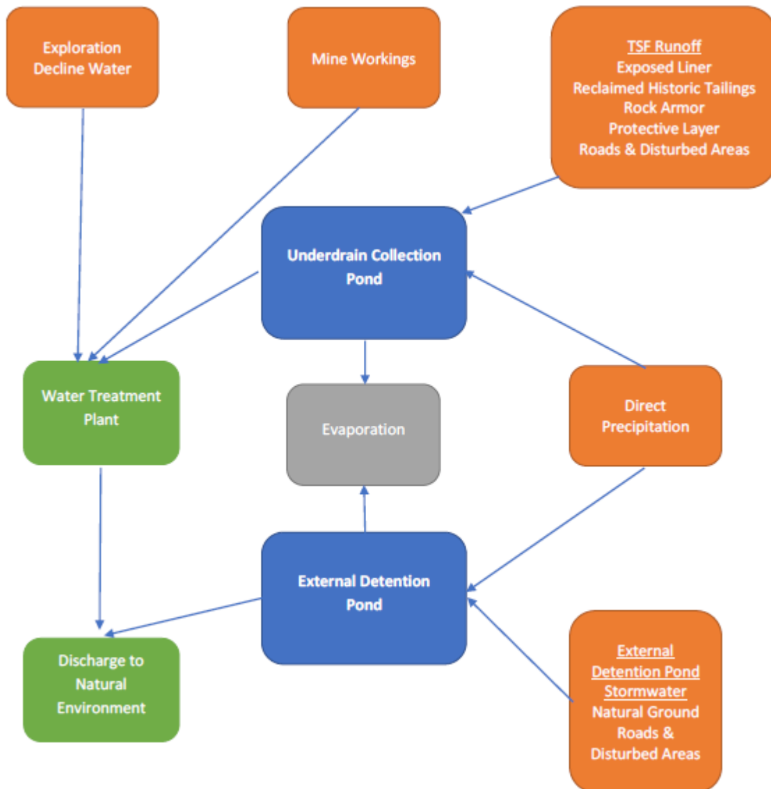
FIGURE 8.1 WATER BALANCE MODEL SCHEMATIC
