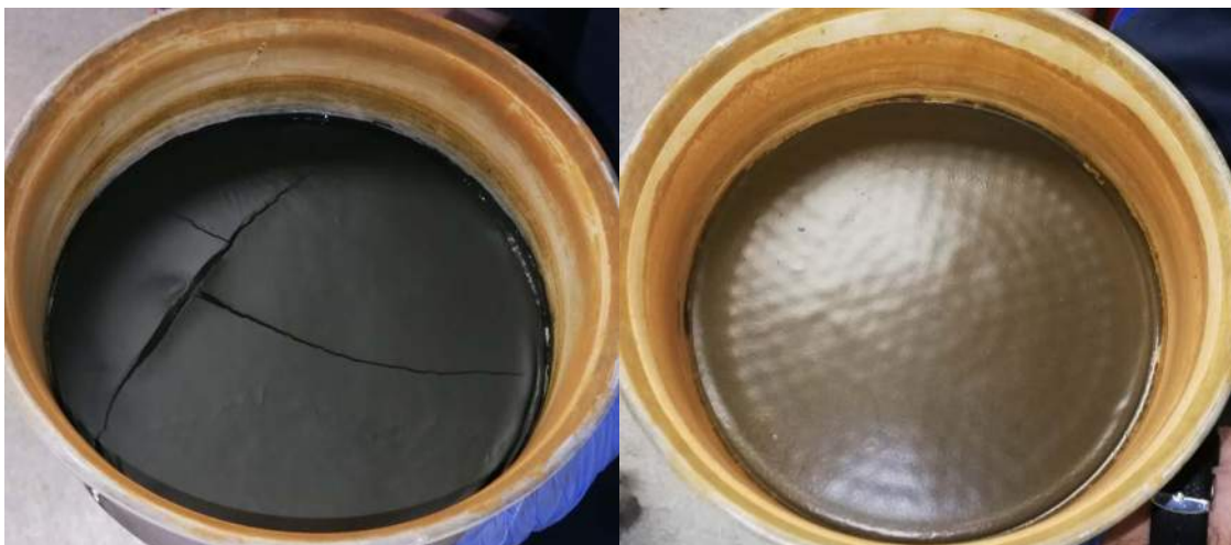
Figure 6-4. Filtered Solids Residue from NF 70% Test Case (Left) and RO 60% Test Case (Right).
