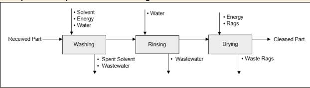
After qualitatively writing down the process, we can list the inputs and outputs and add quantitative values. This is shown in the example input and output table below. For the industrial washer, we know that it takes about 40 gallons of the solvent-based cleaning fluid per part we wash. We can then estimate how much of the input is used annually by multiplying the 40
