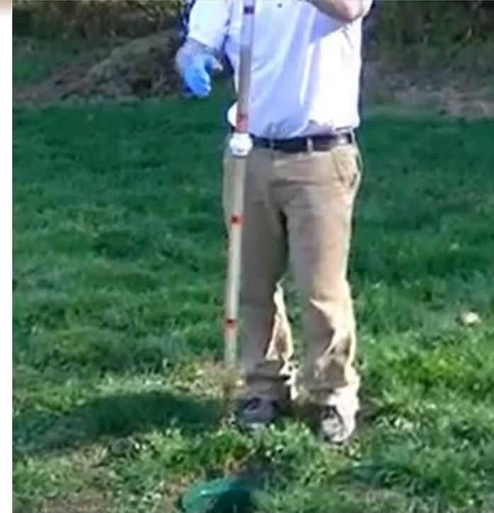
A standard rule of measurement is that you're due for a pump out when the solids (scum + sludge) accumulate to about 30 – 50% of the total volume your tank
