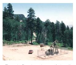
Figure 3. Pumping unit on producing oil well. Note car for scale.
