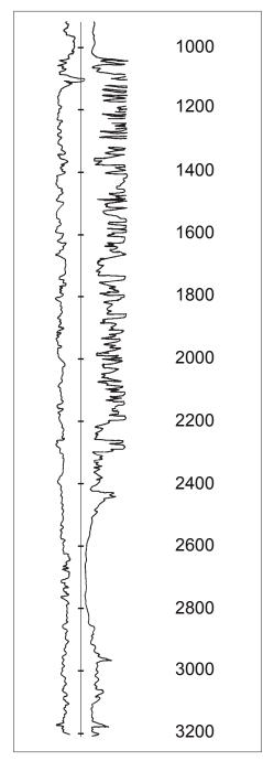
Figure 2. Segment of typical well log. Curve deflections indicate rock properties that can be correlated from well to well. Numbers represent depth in feet below surface .
