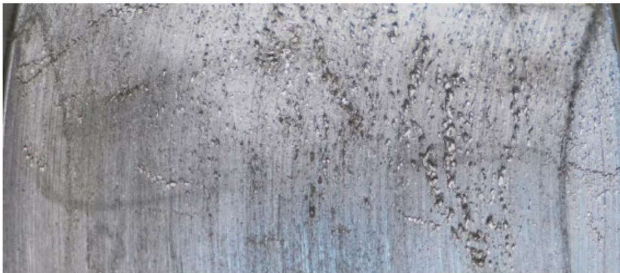
Cavitation Damage to the Pump Casing
