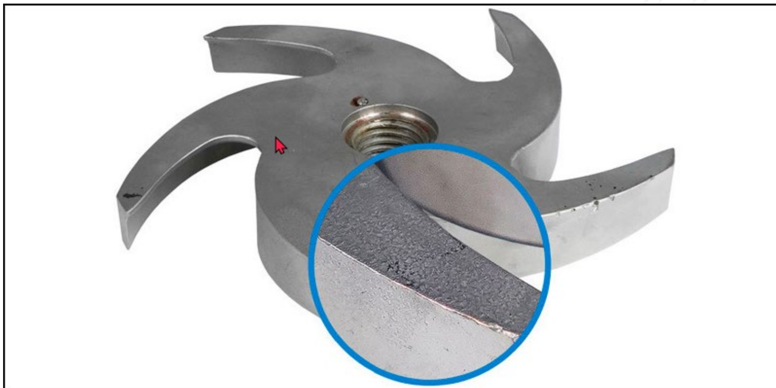
Cavitation damage to the impellor
