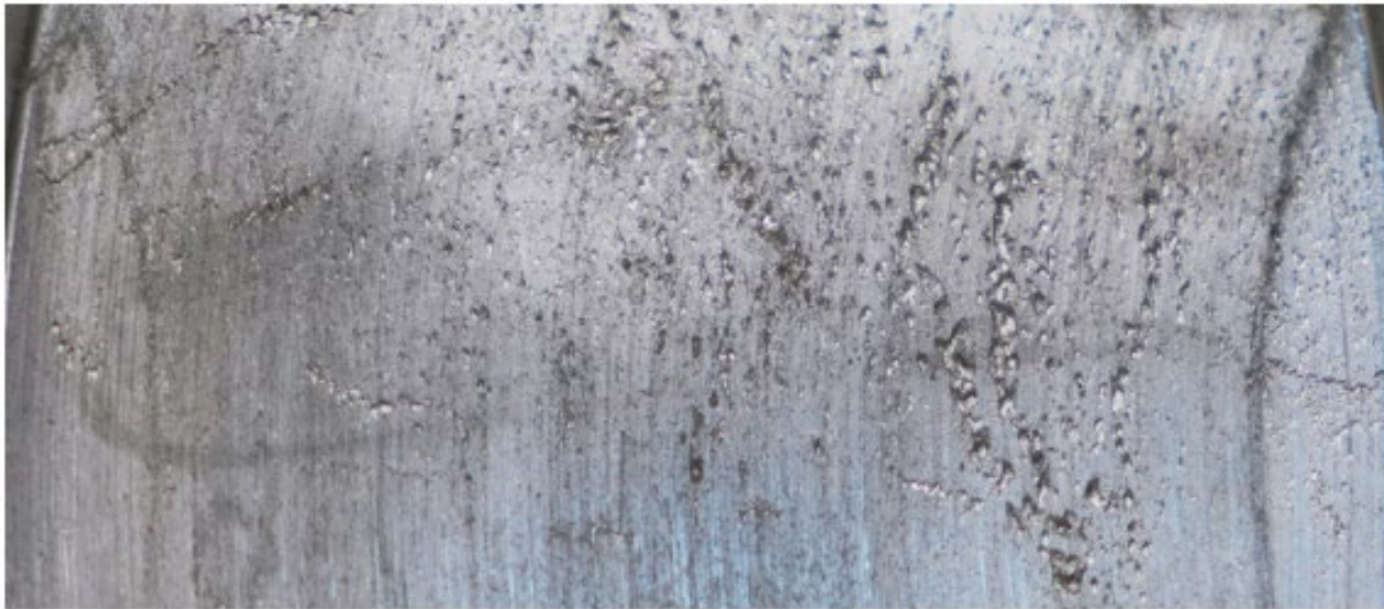
Cavitation Damage to the Pump Casing
