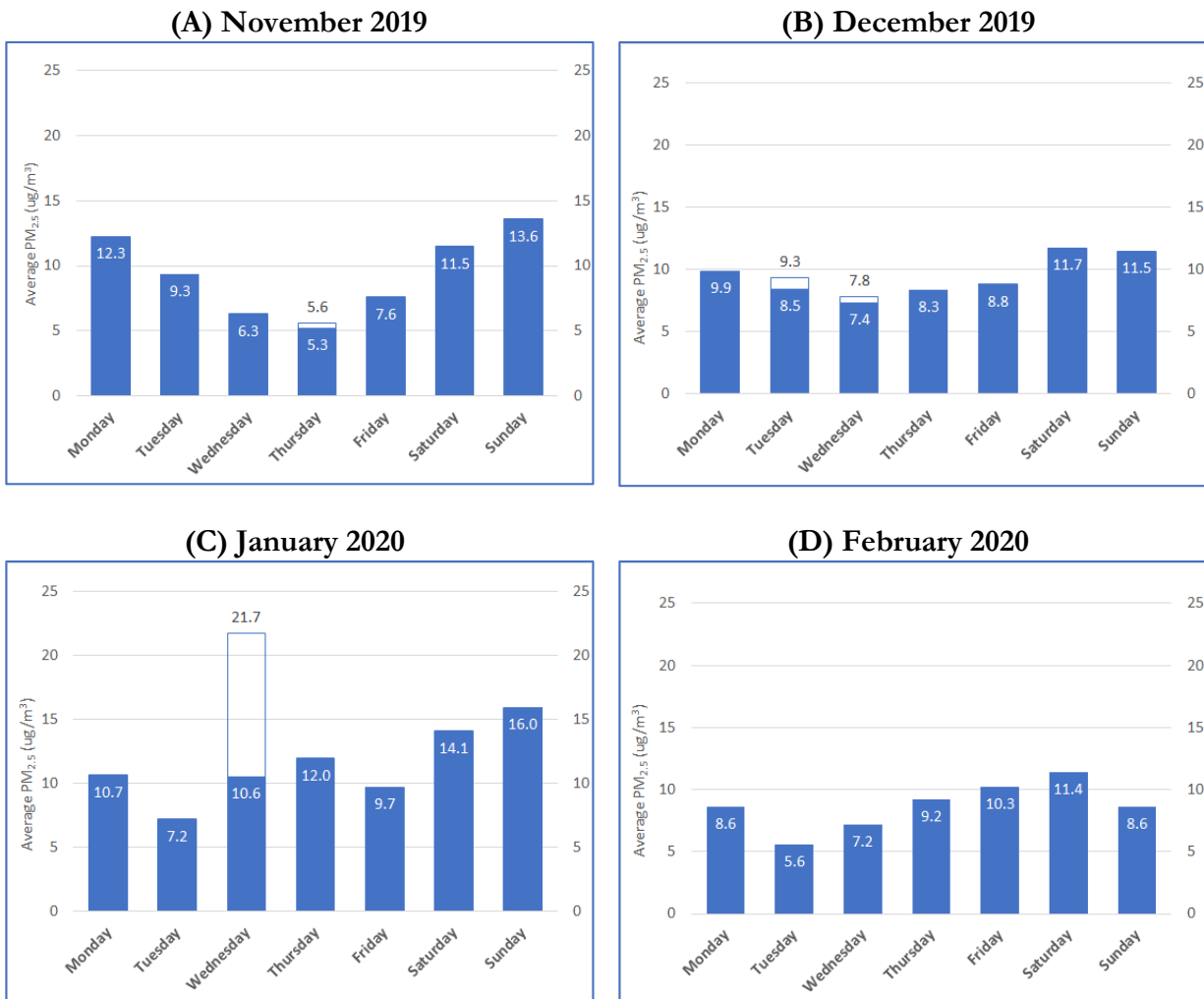
Figure 10. PM 2.5 averaged by month and day of the week for November 2019 (A), December 2019 (B), January 2020 (C), and February 2020 (D). Where appropriate, values are depicted both including and excluding holiday outliers.
