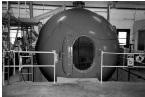
Figure 2. Twelve-foot sphere in which the gaseous products of 2-lb explosive charges are confined for analysis.
