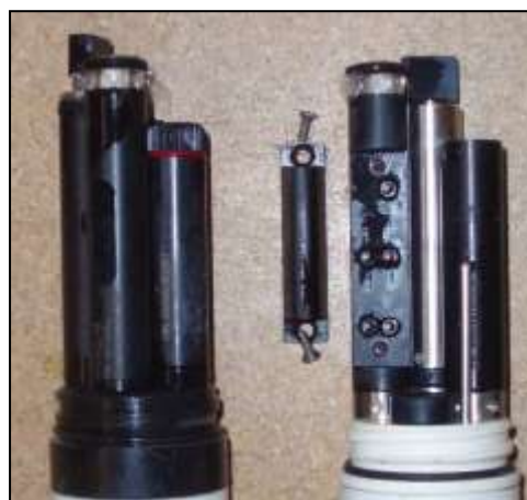
FIGURE 9.3. New graphite conductivity sensor (left). Old nickel conductivity electrodes (right). Both are combined with the DO probe.
