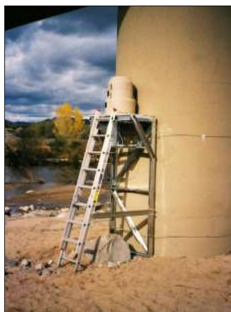
FIGURE 6.3. Example autosampler installation scenarios- under bridge (left) and secured to bridge support (right)
