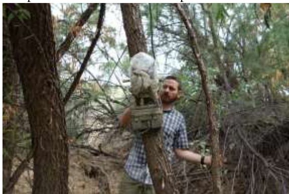
FIGURE 8.20. Place a trash bag over the camera when using spray paint to camouflage the equipment.
