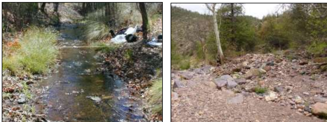
FIGURE 7.11. Left: Bankfull identified by tape measurer at slope break. Right: Multiple bankfull indicators (change in particle size, top of point bar, slope break).
