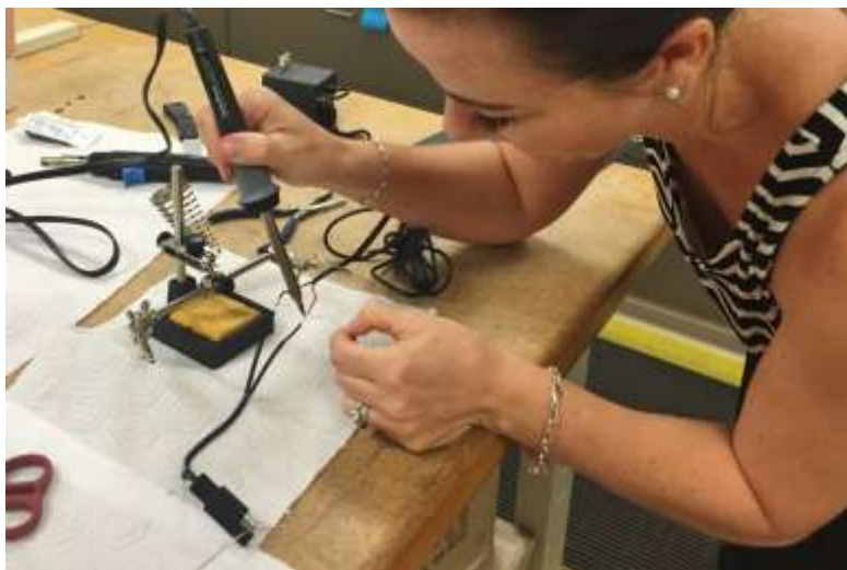
FIGURE 8.5. Soldering and altering the solar panel to connect to the external battery.
