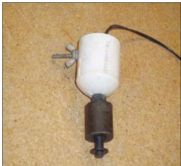
FIGURE 6.5. Float switch (black) connected to PVC cap
