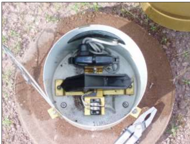
FIGURE 6.1. View of rain gage with funnel and screen removed. Note that the tipping buckets are free of any cables or wires that may hinder them from moving freely.
