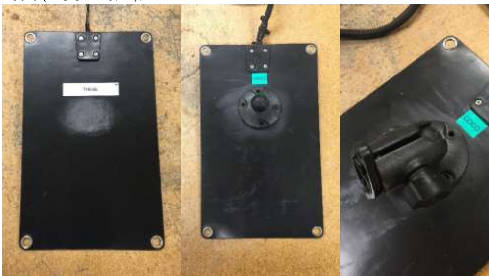
FIGURE 8.11. The solar panel RAM mount attachment process.
