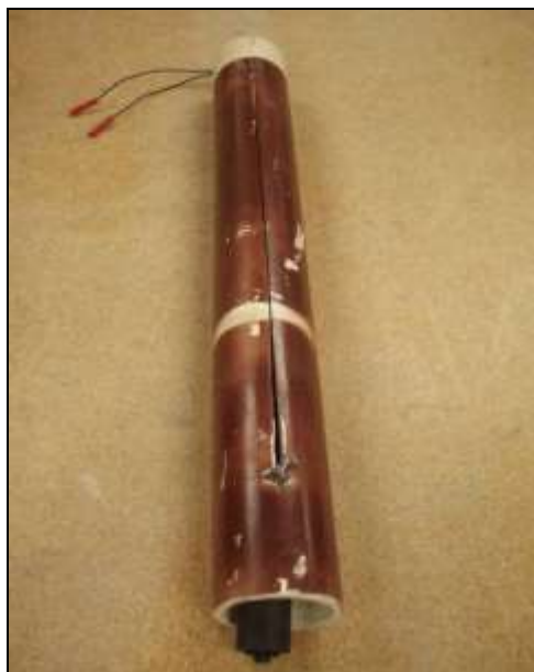
FIGURE H.1. Float switch assembly installed into well screen PVC pipe
