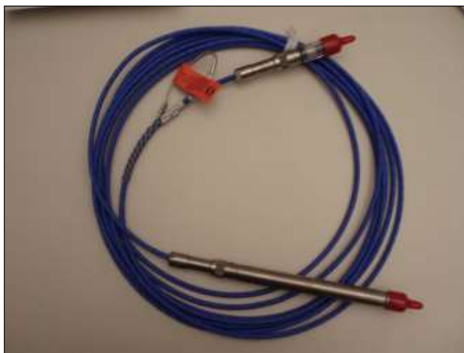
FIGURE 6.9. In-situ Water Level Logger with vented cable attached
