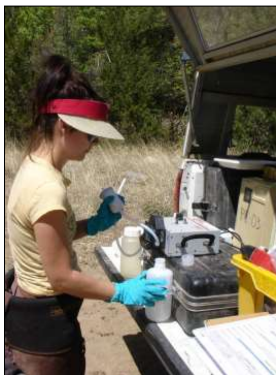
FIGURE 3.7. Filtering set-up. Note the peristaltic pump, tubing, collection bottle, receiving bottle, filter and nitrile gloves.
