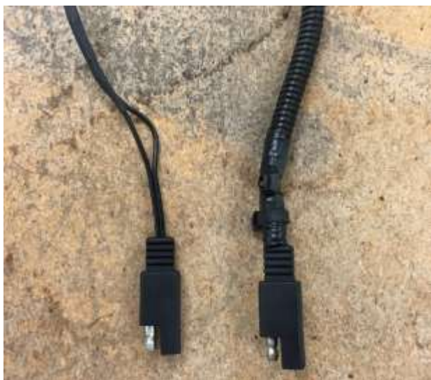
FIGURE 8.12. Comparison of solar panel exposed wire vs. wire with sleeving.
