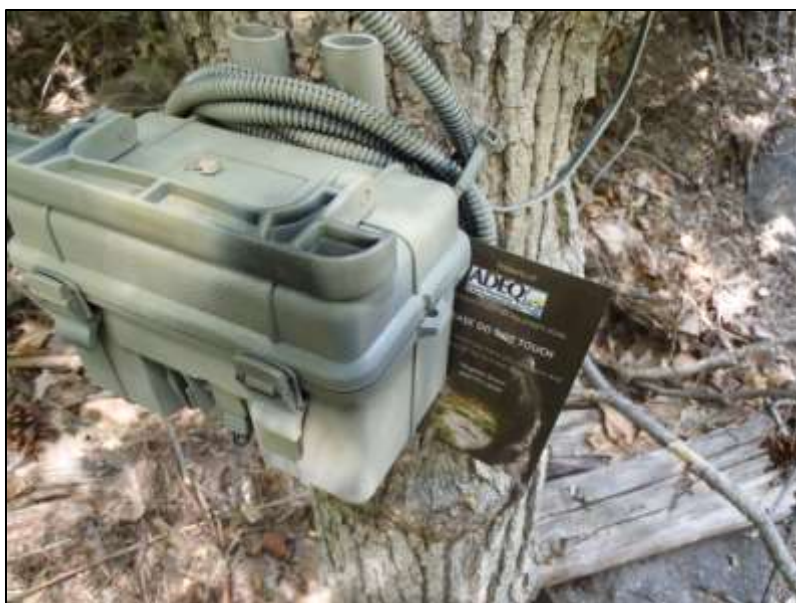
FIGURE 8.18. External battery with solar panel wire wrapped around to avoid rodent chewing.
