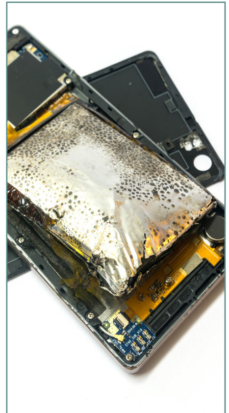
Note: Batteries with damage like this are NOT universal waste.
